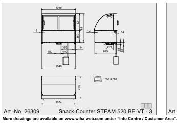
The steam generator operates fully automatically and is equipped with an automatic water filling system. The water tank can be placed under the device in the counter furniture and can be easily removed for daily filling. The humidifier tray of the steam generator can be easily removed for cleaning. It can be cleaned in a dishwasher.
