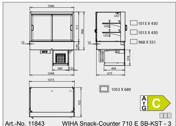
The drawings are shown with special accessory that is not included in the scope of delivery; more drawings are available on [www.wiha-web.com](http://www.wiha-web.com) under "Info Centre / Customer Area".
