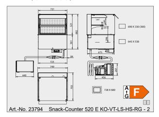
Self-service version that is open on the customer side, recessed cooling pan, front air curtain and sneeze guard. The rear panel is closed. The side glass panes, the upper glass pane and the height adjustable shelves are made of safety glass. For good illumination, a shielded LED light (standard colour: white) is mounted above each shelf. The shelves are suitable for Gastro-Norm dimensions. The mounting lip makes installation
