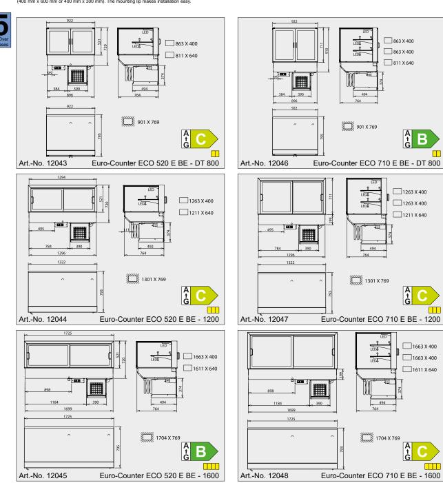
The drawings are shown with special accessory that is not included in the scope of delivery; more drawings are available on www.wiha-web.com under "Info Centre / Customer Area"
